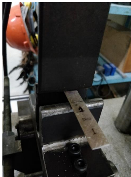
Gambar 3.36 Proses pengujian bending
