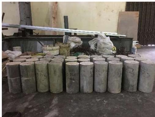
**Gambar 3. 3** Benda Uji Beton
