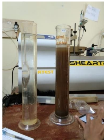
Gambar 3. 5. Pengujian Hydrometer analysis
