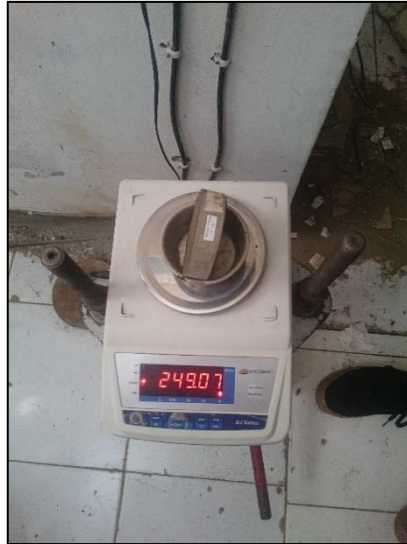
Gambar 3. 4. Penimbangan sampel tanah selesai oven
