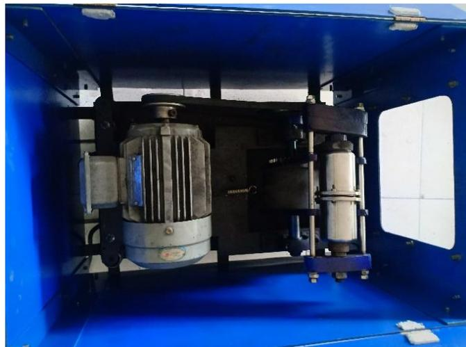
Gambar 2.2 Mesin *Shaker Milling*
