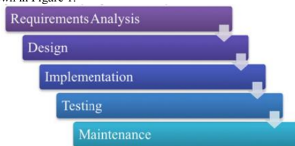
Figure 1. The stages of the Waterfall Model [10]
