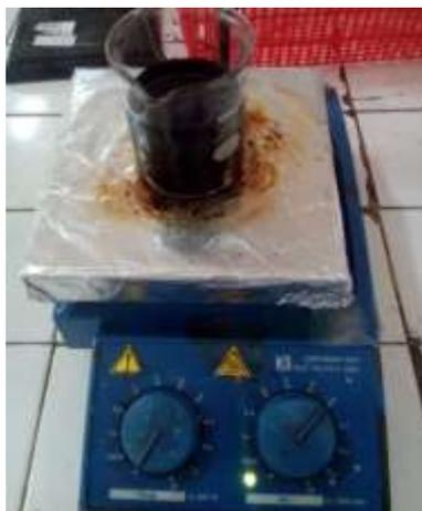
**Gambar 4.2** Proses pencucian reduktif
