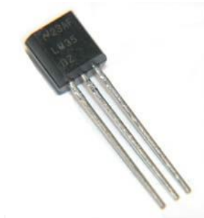
Gambar 5. Sensor Suhu LM 35
