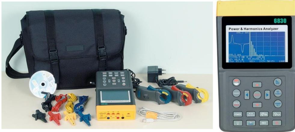
Gambar 3.2 *Power And Harmonic Analyzer* Langlois 6830
