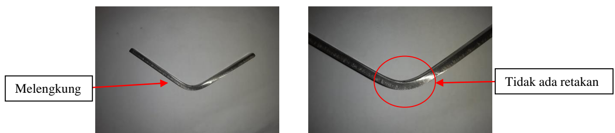
Gambar 4.5 Spesimen Hasil Pengujian Bending Bahan Stainless steel 304
