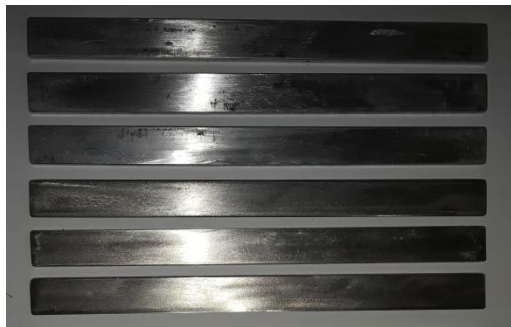
Gambar 3.3 Spesimen Uji Bending Material Stainless Steel 304 dan Aluminium 6061
