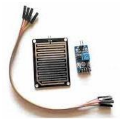
Gambar 2. 14 Grid Impedance Rain Sensor (Marpaung, 2017: 73)
