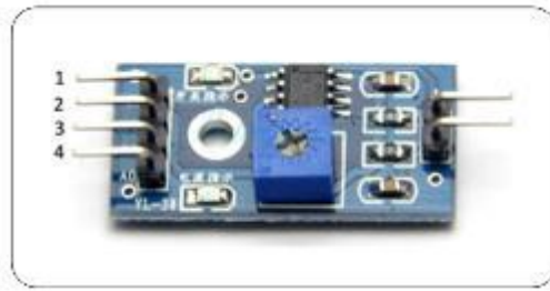
Gambar 2. 13 Modul Rain Sensor (Lestari., 2018: 16)
