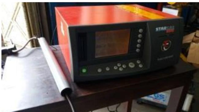
Gambar 2.7 Exhaust Gas Analyzer
