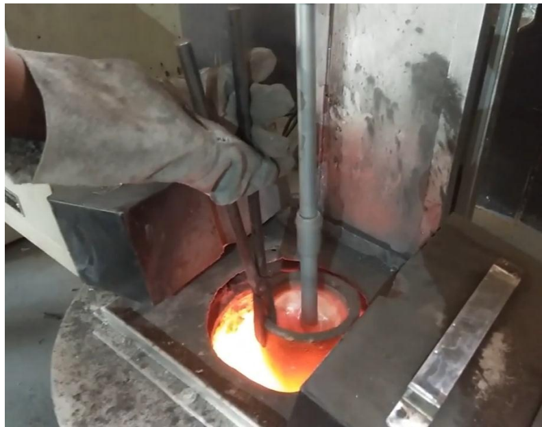
4. Proses Pengecoran Metode Stir Casting
