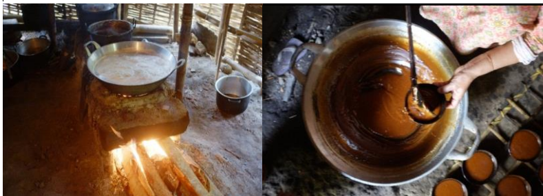
Figure 3. Nira Heating Process,
