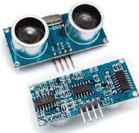
Gambar 2.3 Modul Sensor Ultrasonik
