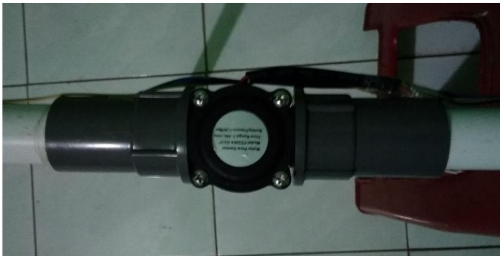
Gambar 4.3 Sensor Aliran Air.
