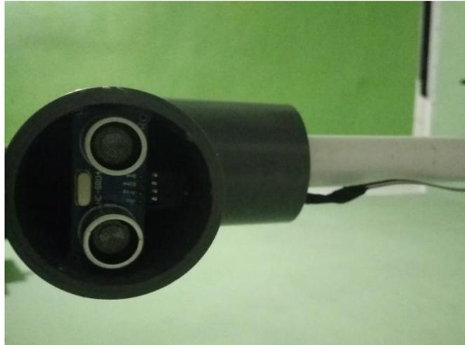
Gambar 4.2 Sensor Ultrasonik
