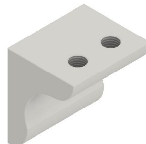
Gambar 4.7 Sub-Assembly Battery Bracket
