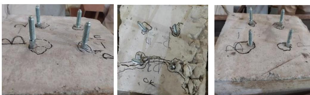
Gambar 4.9. Kegagalan Pasca Pengujian *Post Installed*
