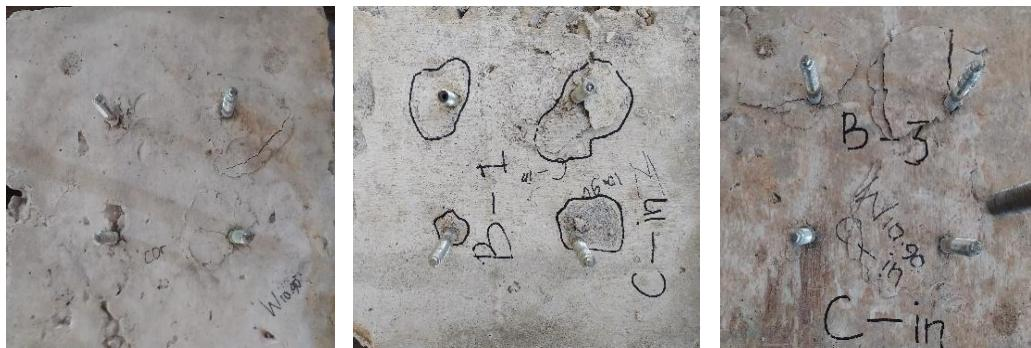
Gambar 4.16. Kegagalan *pullout* angkur secara *cast in place* (Wiguntoro,2020)
