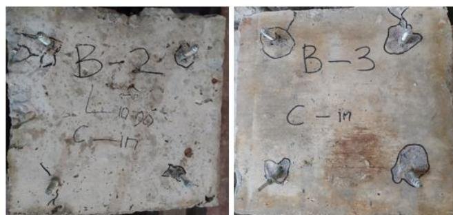
Gambar 4.18. Kegagalan *pullout* angkur secara *cast in place* (Anatasya 2020)
