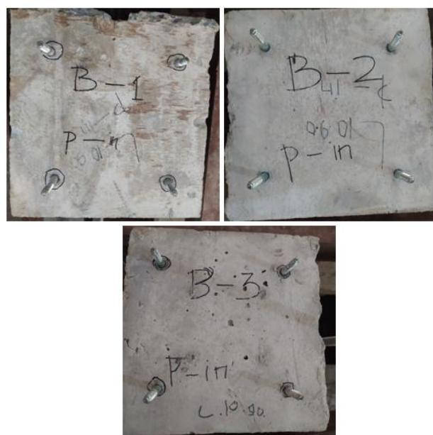
Gambar 4.19. Kegagalan *pullout* angkur secara *post installed* (Anatasya 2020)
