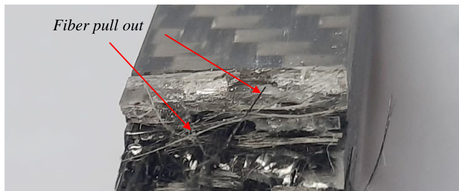
Gambar 4.13 Fiber Pull Out
