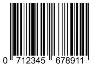
Gambar 2.7 Contoh barcode EAN-13
