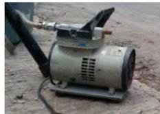
Gambar 3.5 Pompa Vakum
