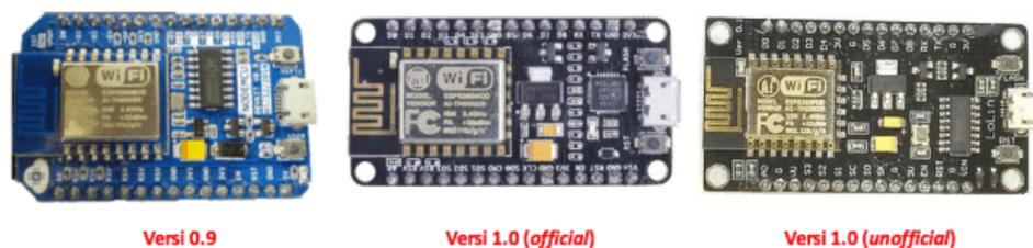
Gambar 2.1 NodeMCU ESP8266
