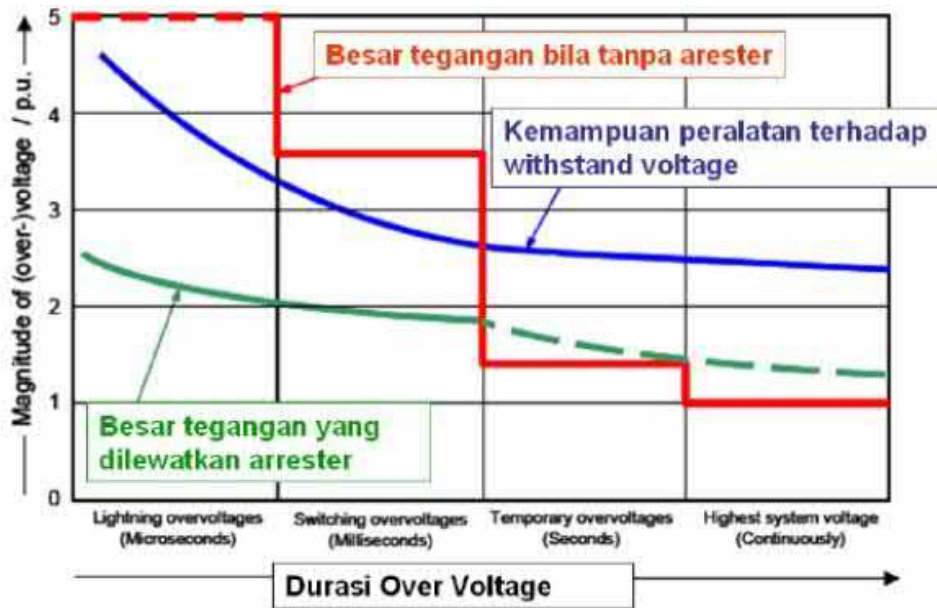
Gambar 2.4 Skematik diagram level tegangan Lightning Arrester Sumber : (SPLN T5.007, 2014)
