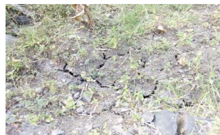
Figure 6. Cracks of the slopes on research location On 2,5 – 5 meter in depth the resistivity value of 6.76 \Omega m is interpreted as clay, on 5 – 15 meter in depth, the resistivity value of 53.8 \Omega m is interpreted as sandy tuffs, and on 15 – 20 meter in depth, the resistivity value of 429 - 3415 \Omega m is interpreted as sandstone. The layer
