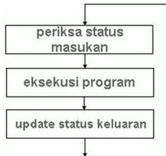
Gambar 2.8 Proses scanning program PLC
