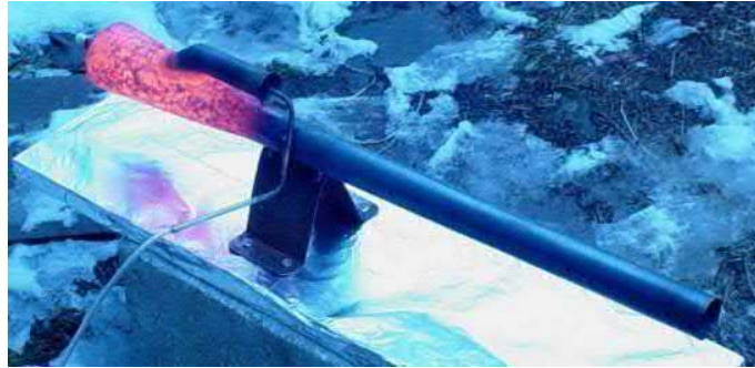
Gambar 2.7. Mesin Focus Wave Energy (FWE) Pulse Jet Engine (Ogorelec, 2005;24)
