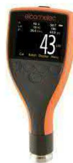
Gambar 2.9 *Dry Film Thickness Gauge*
