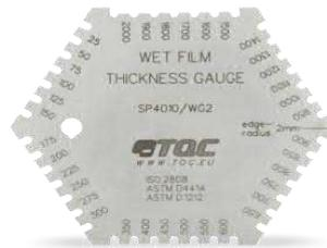
Gambar 2.8 *Wet Film Thickness Gauge*
