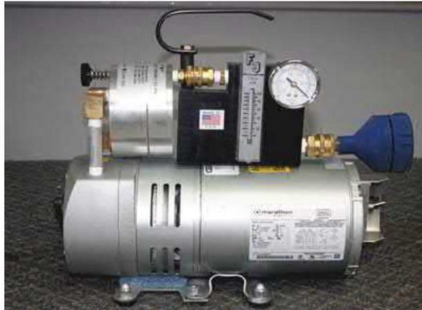
**Gambar 2.4 Low Volume Sampler (LVS)**
