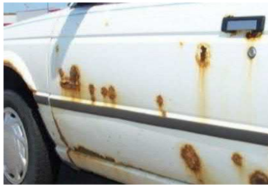
Gambar 2. 13 Korosi Bodi Samping
