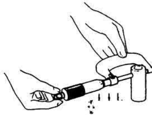
Gambar 2.23 Mengukur Diameter Pen Piston ( Workshop manual engine 4JA1/4JH1 models )
