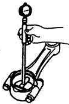
Gambar 2.17 Kerenggangan Poros Engkol dan Bantalan Tangkai Piston (Buku Pedoman Perbaikan Mesin Diesel Isuzu Panther Model c223)
