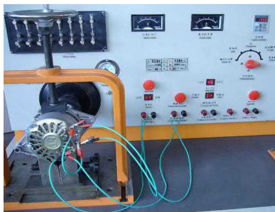
Gambar 2.12. Pengetesan Alternator pada Alternator bench test ( https://indonesian.alibaba.com/product-detail/auto-electrical-test-bench-alternator-starter-motor-test-generator-tqd-model-distributor-477878548.html )
