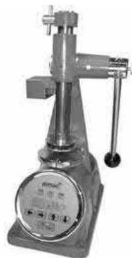
Gambar 2.5 *Valve Spring Tester*
