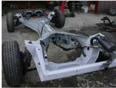
Gambar 2.4. Chassis tipe backbone tube (Wakeham, 2009: 42)
