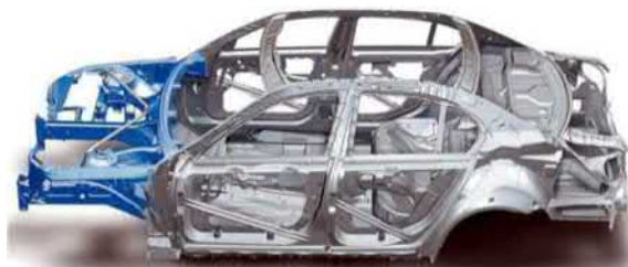
Gambar 2.5. Chassis tipe monocoque (Lombogia dan Siahaan, 2016: 2)
