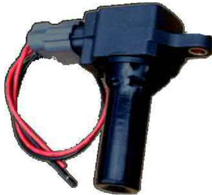
Gambar 2.8 Progressive ignition coil racing generation / koil R9 (Babad150f, 2010).
