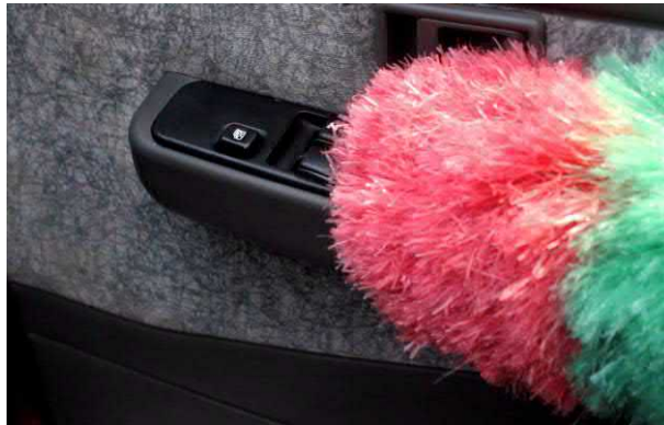
Gambar 2.35. Pembersihan sakelar power window
