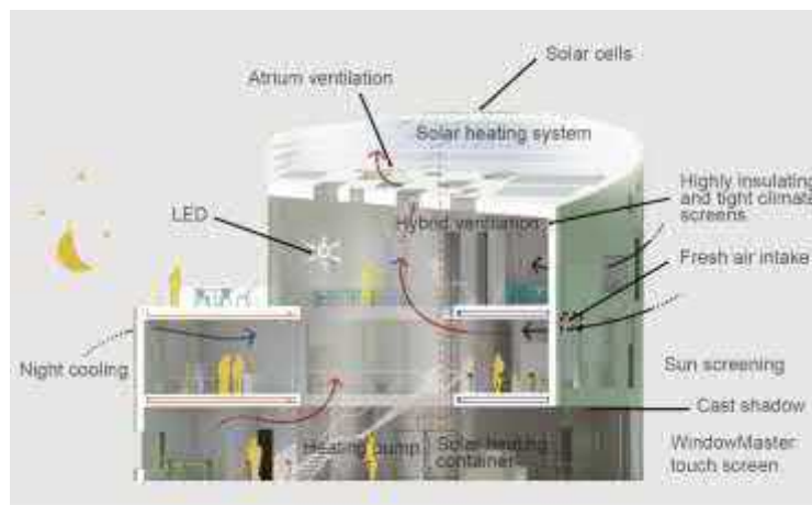
Gambar 2.55. Green Lighthouse Section
