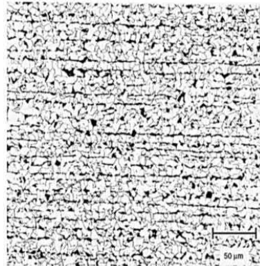
Gambar 2.7 Struktur mikro ferit (ASM International, 2004: 1440)
