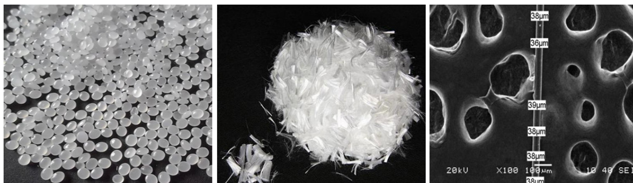
Fig. 1. Photograph of a) HDPE pellets; b) PVA fiber; and c) SEM image of single PVA fiber
