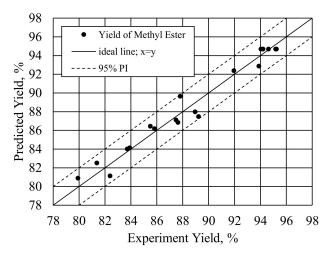
Fig. 1 The correlation between the predicted value and experimental value of biodiesel yield ( $R^2 = 0.9701$ ) with 95 % of Prediction Interval (PI).
