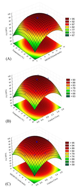
Fig. 2 The 3D response surfaces profile of methyl ester yield as affected by independent variable
