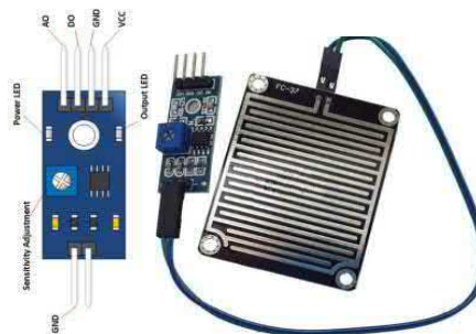
Gambar 2.17 Konfigurasi sensor hujan ( https://sc01.alicdn.com/ )
