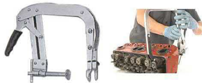
Gambar 2.48. Valve Spring Compressor (Sumber : Efendi, 2013)
