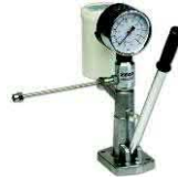
Gambar 2.47. Diesel Injector Tester (Sumber : Efendi, 2013)
