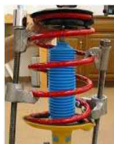
Gambar 2.52. Coil Spring Compressor (Sumber : Efendi, 2013)
