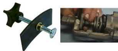
Gambar 2.51. Disc Brake Piston Compressor (Sumber : Efendi, 2013)
