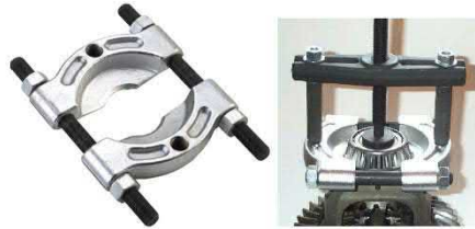
Gambar 2.39. Bearing Puller Attachment (Sumber : Efendi, 2013)
