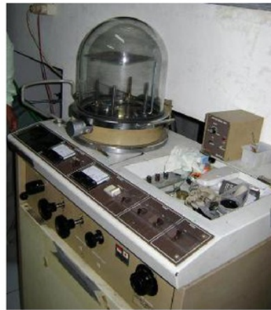
Gambar 5.11: Vakum evaporasi (VE) Model JEOL JEE-4X
