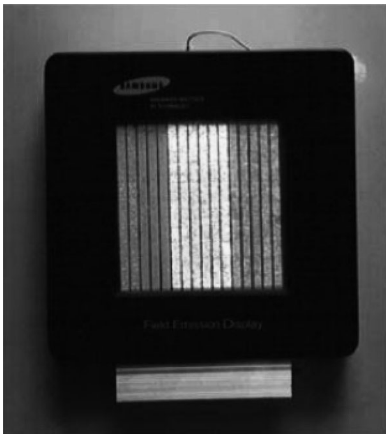
Fig. 11 A prototype 4.5-inch field emission display fabricated by Samsung using CNTs (Adapted from [60])
