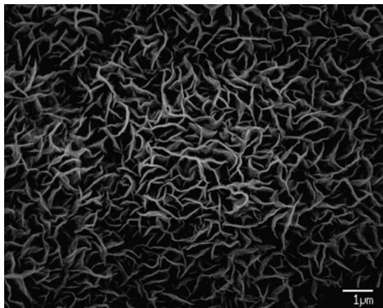
Fig. 12 Carbon nanowalls grown in the MW PECVD as described by Chuang et al. [138, 139]
