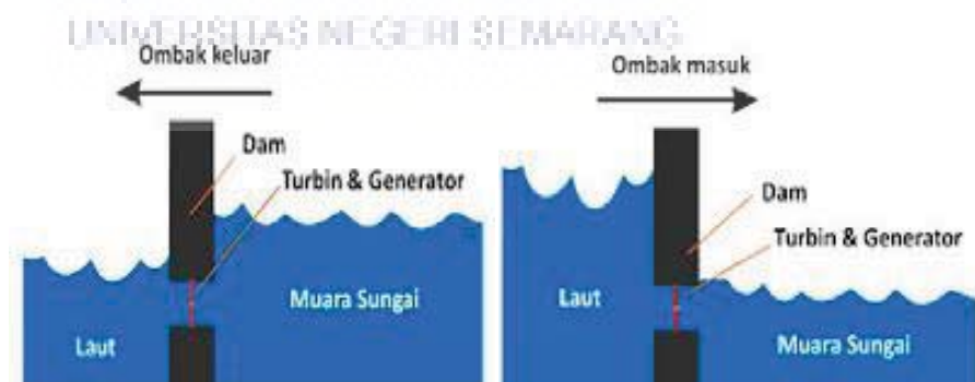
Gambar 2.1 Prinsip Kerja Barrage Tidal System Sumber http://osy.org/education/WaterPower
