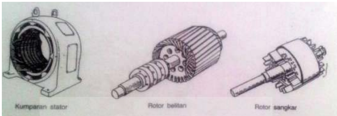
Gambar 2 1 kumparan stator, rotor belitan, rotor sangkar (Dasar Tenaga Listrik 1989)
