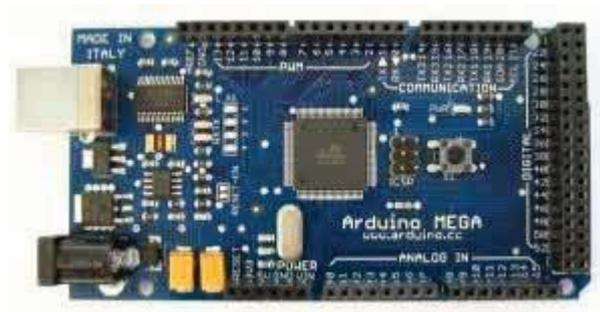
Gambar 2.2 Arduino Mega
