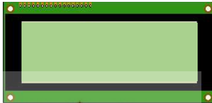
Gambar 2.5 LCD dot matrix 20 x 4
