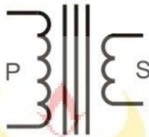
Gambar 2 Simbol Transformator Step Down
