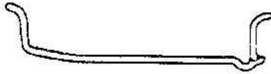
Gambar 14. Flat Base Rim ( https://mardiyan22.files.wordpress.com/2011/01/ban-dan-roda.pdf )
