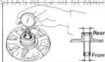
Gambar 2.40 Memeriksa Stator Shaft Bushing (Novriza, 2012: 46)
