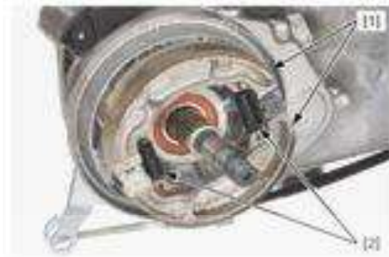
Gambar 21. Melepas Kanvas Rem (Astra Honda Motor, 2012: 17-5)
