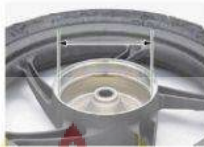
Gambar 19. Mengukur Diameter Dalam Tromol (Astra Honda Motor, 2012: 17-5)
