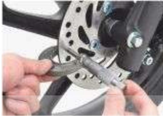
Gambar 40. Memeriksa Ketebalan Cakram (Astra Honda Motor, 2012: 17-11)
