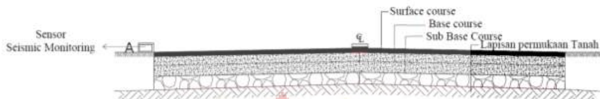
Gambar 4.7. Perletakan alat sensor seismic monitoring
